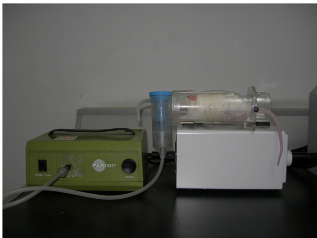
Fig. 2. “Nose-only” inhalation apparatus used for administering inhalable Ins–SLNs to rat.
